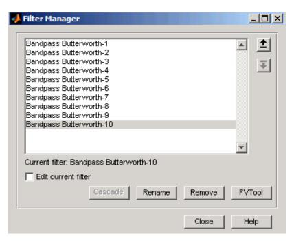
Press Ctrl+click on each filter name to select all the filters, and then click FVTool. FVTool opens with the filter responses overlaid for easy comparison. (If you want to view a single filter in FVTool, click the Full View Analysis button when that filter is shown in the app's display panel or select View > Filter Visualization Tool).
