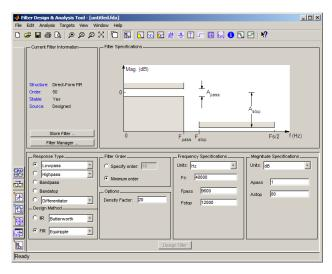
The bottom half of the app shows the Filter Design panel, where you specify the filter parameters. Other panels, such as Import filter from workspace and Pole/Zero Editor, which you access with the buttons on the lower left, are also displayed in this area. If you have other products installed, you may see additional buttons.
